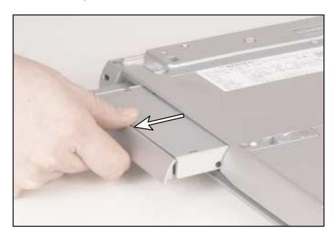
**9** Firmly push the secondary battery straight into the bay until the latch clicks into place.
